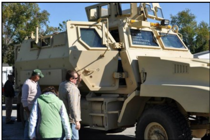
Checking out the MRAP - Capable of traveling in up to 4 feet of water or deep snow.
